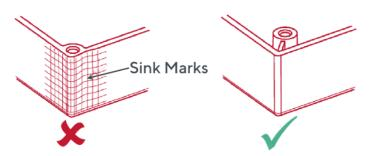
Different materials also have different shrink rates. When designing parts for injection moulding, you usually draw the part to your desired dimensions, however then cut the mould cavity in the tool slightly larger to account for the shrinkage. This is why you need to know the material you want to mould your product in prior to constructing tooling as it is difficult to change material and keep the desired original dimensions.
