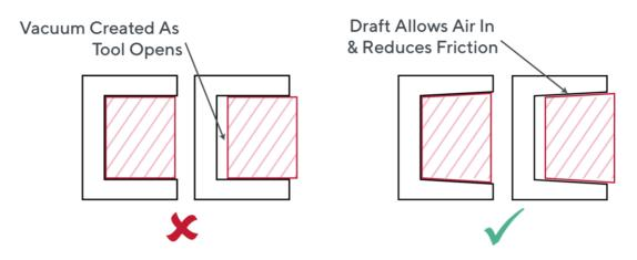
Draft is further required when applying textures or adding embossed or debossed lettering or logos to a plastic component. Draft for textures varies depending on the texture, however a good rule of thumb is to add an additional 1.5° of draft for every 0.025mm depth of texture.
