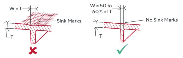
Where ribs intersect, the intersection should be cored out so that a thick point is not created. Ideally, these cores should have a diameter of 5mm or greater.
