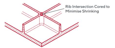
Further, rib height should be limited to 3 times the nominal wall thickness of the product. Ribs should be spaced a minimum 2 times the nominal wall thickness apart.
