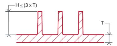
It is important to remember that with injection moulding, where there isn't plastic, there is steel, and this steel must be able to cool and it can't be too fragile – you can't have a really long, thin piece of tooling steel as it simply won't last the repetition, heat, and forces of the injection moulding process.
