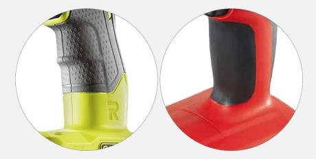
Noticeable join/assembly lines are indicative of components trying to be manufactured cheaper. However, this isn't necessarily a bad thing, particularly for power tools which will be used outside, and will likely suffer damage and still need to be usable. This noticeable join could be resultant from several things, such as:
