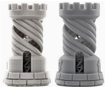
Image 2: FDM (Left) vs. SLA Surface Quality (Right)
